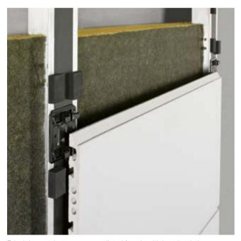
Principle: curtain-type, rear-ventilated facade with heat insulation
